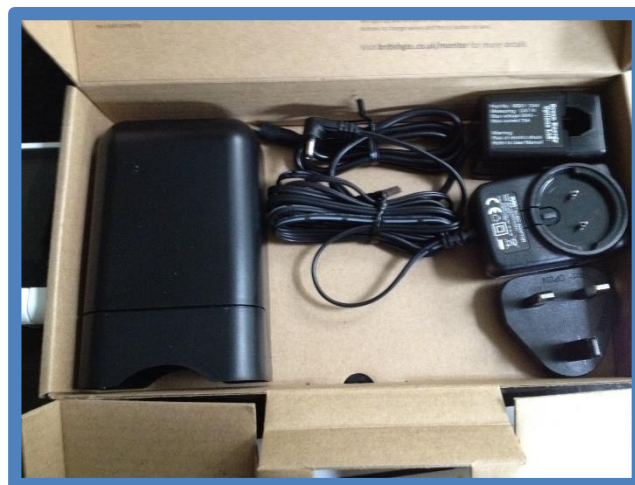
Figure 2: The transmitter (left), sensor (top right) and power supply (middle and bottom right)
